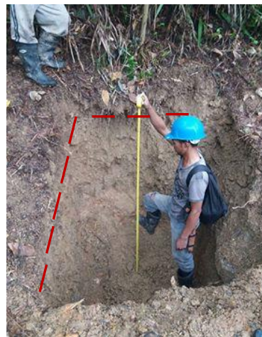
Figure 7. A) Red lines showing dimensions: Width- 1.4m, Length- 1.7m, Height- 1.7m B) From top to 1.2m, sand with clay, brown C) 1.2m to 1.7m, oxidized, clay-chlorite altered andesite porphyry (pebble to cobble size) (MGB XI, 2018)
